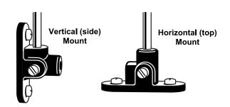
The J-Base is a glass reinforced polycarbonate fixture for mounting WindTrak to side, top or front of masts on most small boats and dinghies.
